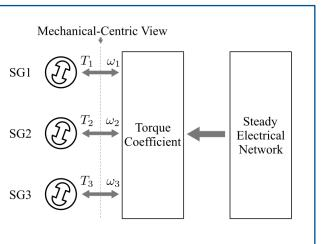
Mapping dynamics through ports can be used to form composite, unified system models.
