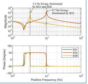
Torque coefficient of each machine can can be found from element of transfer function matrix G"
