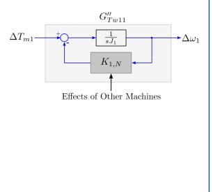
Imaginary part of torque coefficient is synchronizing torque Real part is damping torque
