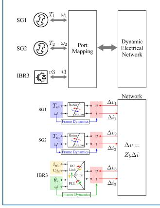
Electrical-centric analysis found in inverter-based microgrids.
