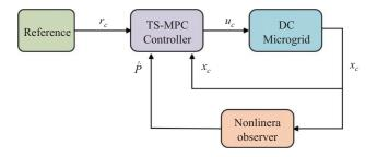
Fig. 4. DC microgrids control layer and a state estimation.
