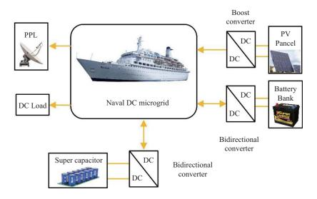
Fig. 1. A model of naval DC microgrids.
