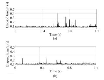
Fig. 7. Time spent on computation for each optimization process. (a) NL-MPC. (b) TS-MPC.
