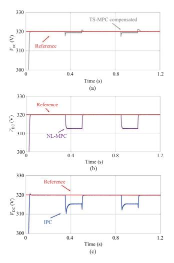
Fig. 8. Performances of DC link voltage for each approach. (a) NL-MPC. (b) TS-MPC. (c) IPC.
