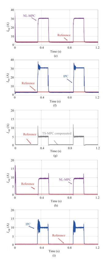
Fig. 6. Performance of DC microgrids using the TS-MPC, NL-MPC, and IPC control methods with a pulse load of 4 kW. (a) TS-MPC compensated. (b) NL-MPC. (c) IPC. (d) TS-MPC compensated. (e) NL-MPC. (f) IPC. (g) TS-MPC compensated. (h) NL-MPC. (i) IPC.
