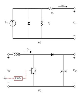
Fig. 2. PV panel model. (a) The equivalent circuit of a PV cell. (b) Connecting the PV panel to the grid.
