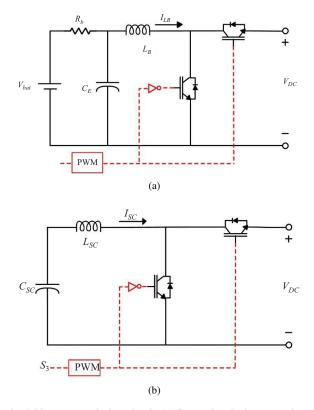
Fig. 3. ESS system equivalent circuit. (a) Connecting the battery to the grid. (b) Connecting the super capacitor to the grid.
